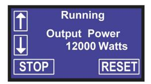
In normal operation the Powersync II will show the status as "Running" and will display the instantaneous Output Power in Watts. Other operating modes that may be indicated are as follows:
