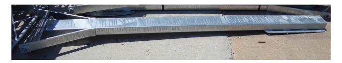
3. Tail Boom: 145 lbs, 13" x 114" x 24" (HxWxD)
