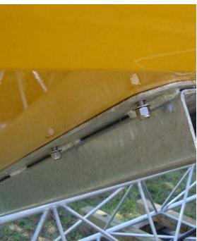
2. Shortly before the crane is scheduled to arrive, attach the tail fin to the tail boom using the hardware provided in the Tail Assembly Hardware Kit. Lay the tail boom on a work surface with the fin mounting plate upward. Position the tail fin on the mounting plate, with the trailing edge bend upward. Eight bolts (3/8"-16 x 1"), 16 flat washers and 8 nylon lock nuts are used. Recommended torque is 20 ft-lb. Set the tail assembly aside for later use.
