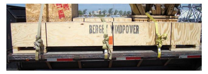
2. Blade Carton: 180 lbs, 16" x 131" x 14" (HxWxD) a. Three rotor blades
