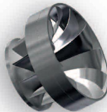
These impulse turbines for the high head range (relatively small discharge with heads of more than 30 m) are manufactured by Geppert with 1 to 6 nozzles. The jet units are offered external and internal controlled.
