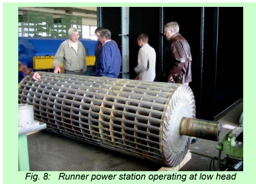
Fig. 8: Runner power station operating at low head
